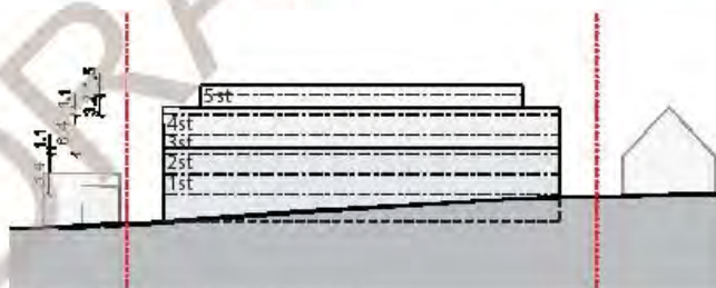
Figure 1.04 - Marion Street - Building envelope - Section A-A
