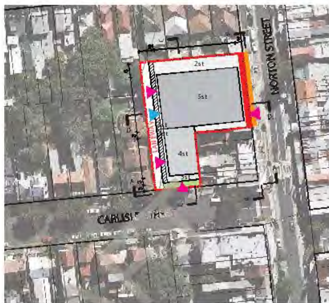
Figure 2.06 - Norton Street Site 3 - Building envelope plan
